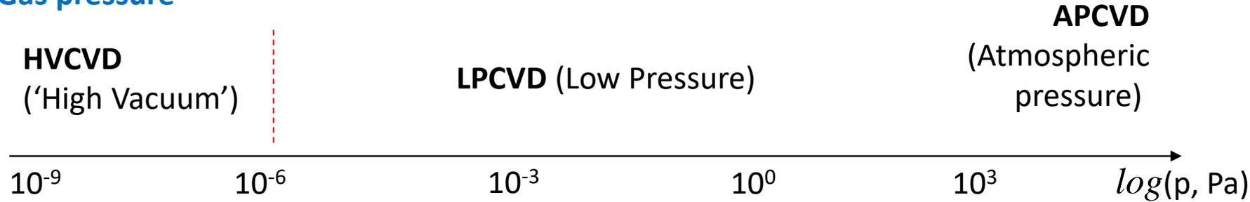
Complexity of the reactor is higher for lower pressure, technologically realistic CVD is mostly atmospheric pressure
