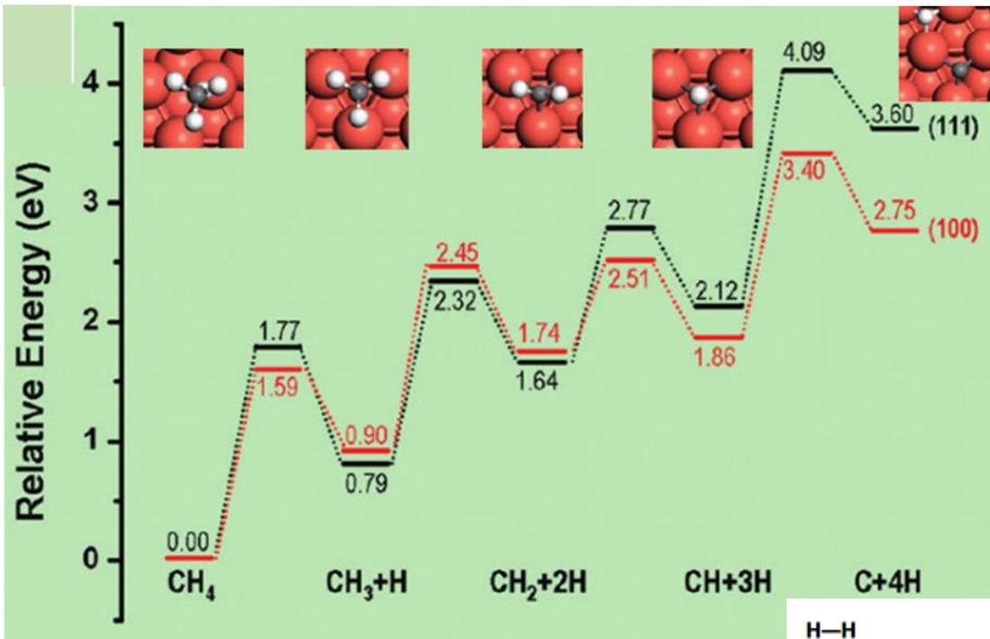
Activation energy results from energy barrier, which can be roughly estimated from quantum chemistry (example for Cu(111) <black> and Cu(100) <red> surfaces)
