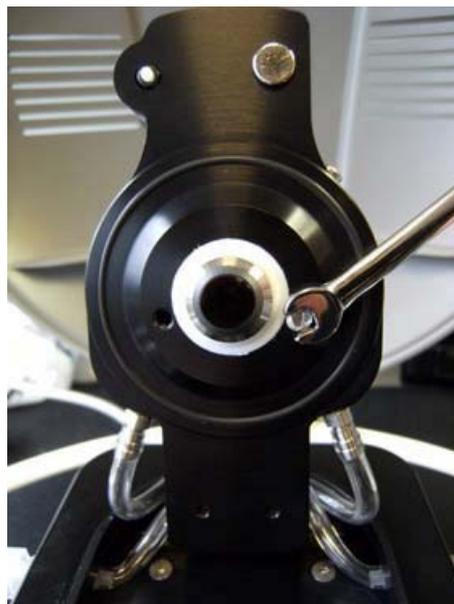
*Unscrew both fluid stopper with supplied wrench*
