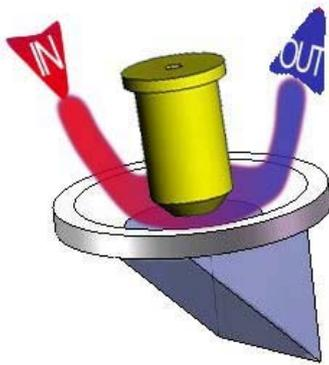
*The flow enters the measurement cell through a first nozzle. When the cell is fulfilled, the flow gets out through a second nozzle. Moving the DTC Up to Down catches a very small sample (few tens of microns thin film layer). The flow keeps going all around the DTC without disturbing the measurement in progress.*
