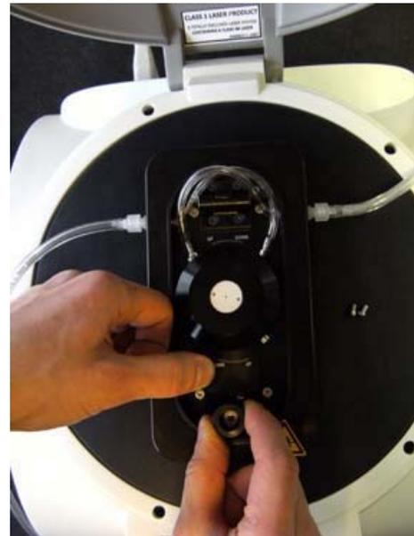
*Hardly press the lever down before turning the closing screw*
